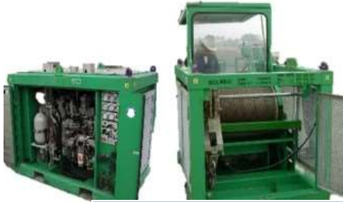
Closed loop winches with 0.108"/0.125" wireline (ASEP)
