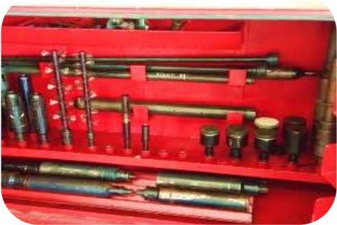
Standard wireline tools for 5" completion
