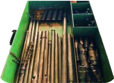
Standard wireline tools for 3" completion
